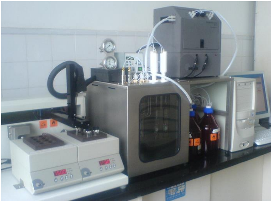
RPV High Temperature Polymer Viscometer with auto sample loading – two measuring positions (second reaction block is optional)
